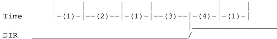
For step type 1, timing parameters 1, 2, and 5 are used. The following timing diagram shows the output waveforms, and what each parameter adjusts.
